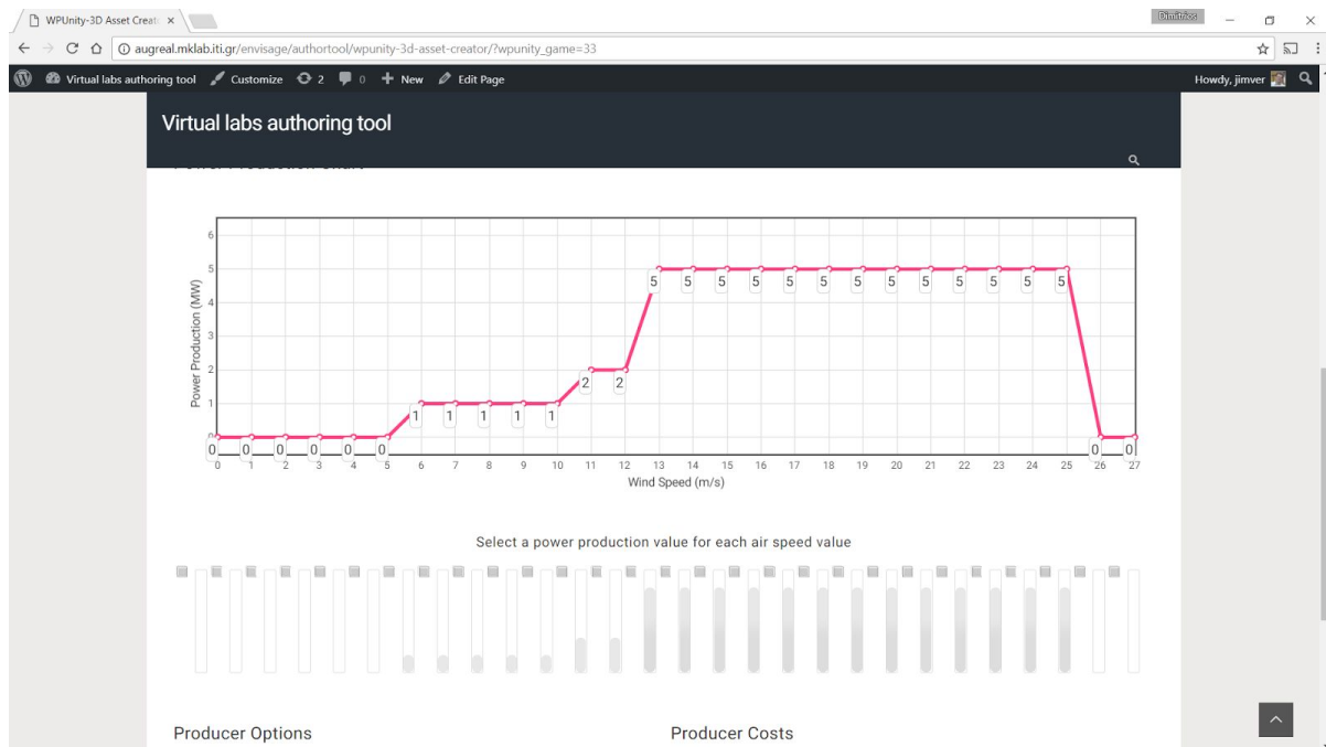
Figure 3.16: Power efficiency curve of the wind turbine. X axis is the Wind Speed, whereas y axis is the power production.
